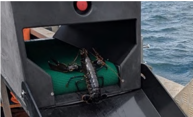
From catch to computer: every animal is scanned to create a detailed 3D model that can be measured automatically. Left: lobster being scanned using Merra-scan. Right: annotated 3D scan of a lobster. Credit Vicki Balfour.
